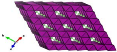
Spinel \text{LiMn}_2\text{O}_4 4.2 V vs. \text{Li}^+/\text{Li}^0
